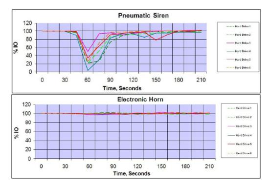
Many codes and standards recommend deenergizing equipment prior to clean-agent discharge. NFPA 75, <u>Protection of Information Technology Equipment</u>, states that "the power to all electronic equipment shall be disconnected upon actuation of a gaseous agent total flooding system ..." This will allow the disk drives to "park," greatly reducing the chance that data will be lost or that disks will be damaged.
