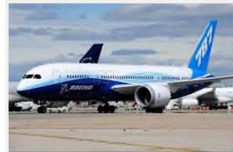
A major goal of Boeing in the development of the 787 was to improve fuel efficiency. Boeing intended the 787 to be 20% more fuel-efficient than the 767 airliner it was replacing. To achieve this objective, Boeing used carbon composite materials as the primary material in the construction of the 787's airframe, significantly reducing the weight of the plane.
