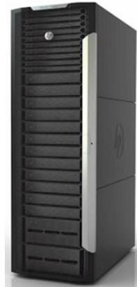
As in the earlier NonStop systems, disk and communication I/O are provided by CLIMs (CLuster I/O Modules). Up to 56 CLIMs can be configured in one system. A communication CLIM can handle four 10GbE Ethernet channels and one 1GbE Ethernet channel. A storage CLIM can support 100 SAS hard disk drives or solid-state disk drives. It can also support Fibre Channel connectivity for SAN attached storage (such as HP XP7 and HP XP P9500 storage subsystems), LT06 tape drives, and virtual tape.
