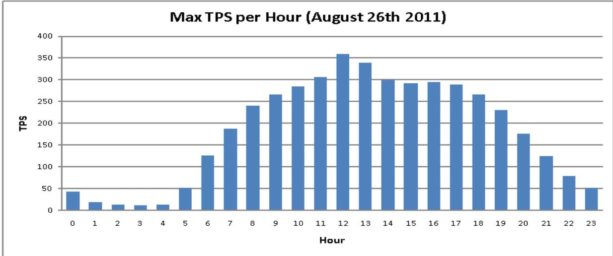
Given the day above a CPU failure in hour 12 or hour 13 could impact the service as we may not have adequate capacity to process the modeled workload comfortably, this is illustrated below:
