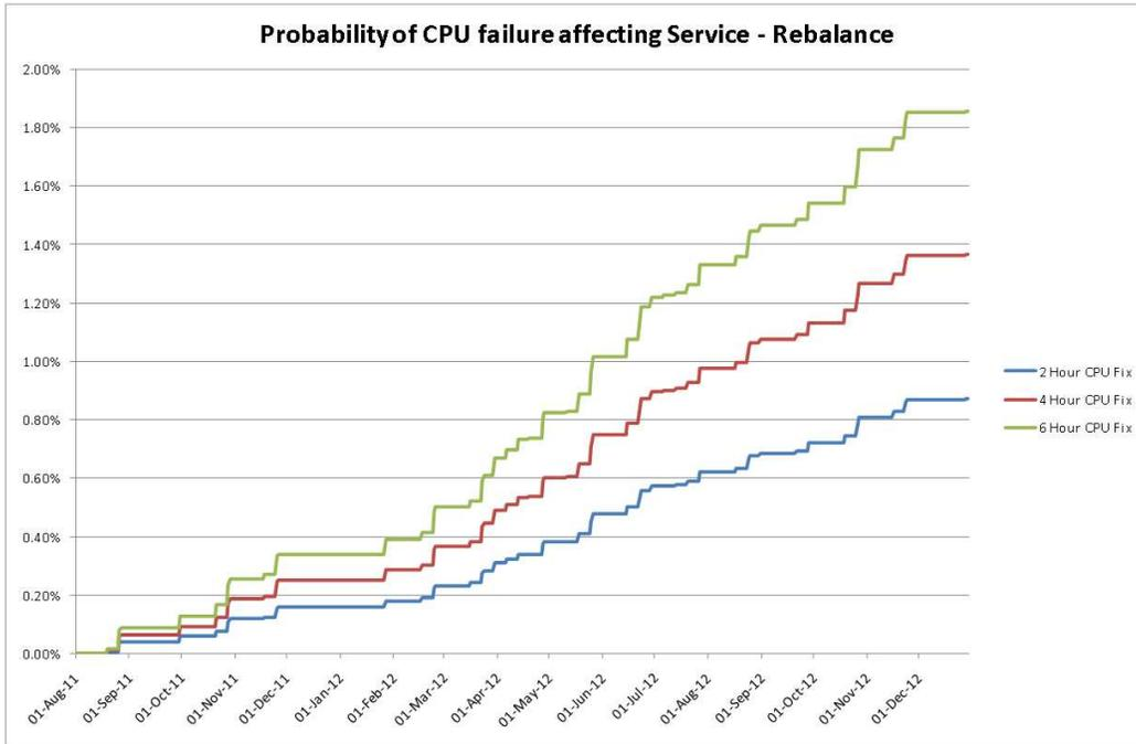
For this option the probability of a CPU failure impacting service over the coming 16 months using a 6 hour fix time is circa 1.85%
