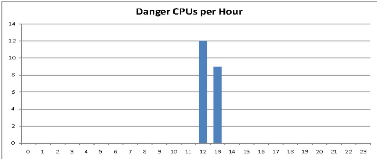
The chart also indicates the number of danger CPU's during each hour, essentially this is taking into account that the system is not perfectly balanced and that the impact of each CPU failing is different. As can be seen when volume reduces in hour 13 the number of danger CPU's also reduces.
