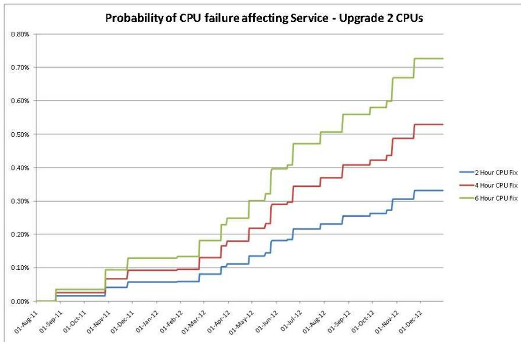
For this option the probability of a CPU failure impacting service over the coming 16 months using a 6 hour fix time is circa 0.7%
