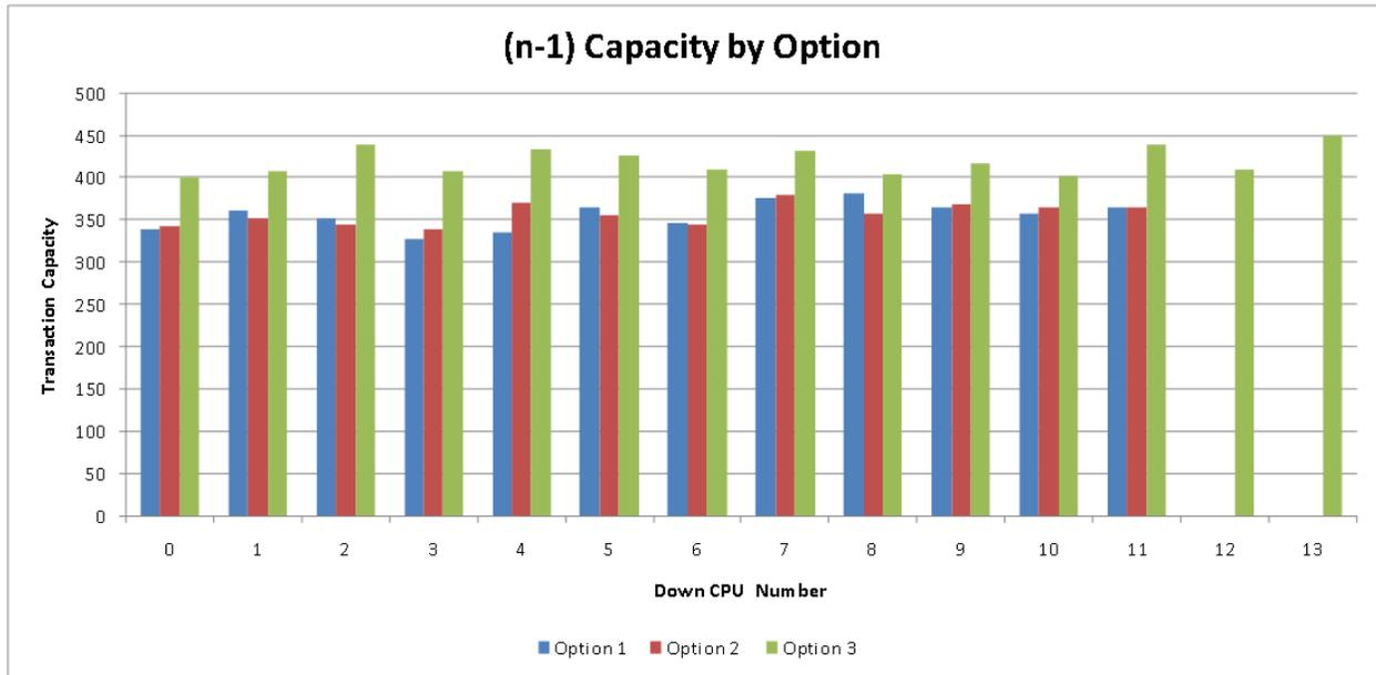
The model illustrated so far takes many factors into account to determine maximum system capacity. For a Production / DR configuration the maximum capacity is that of the system with a single CPU down (n-1) and with none of the remaining CPUs running in excess of 80% utilized.
