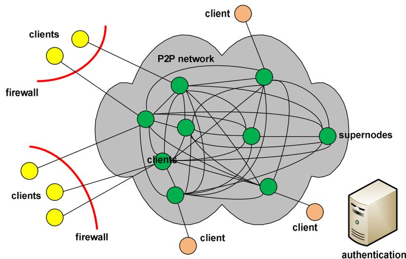
The other function provided by the supernodes is connection of clients behind firewalls. If both clients involved in a connection are behind different firewalls, they cannot communicate directly with each other. Rather, a supernode is assigned to act as a relay node for the connection.
