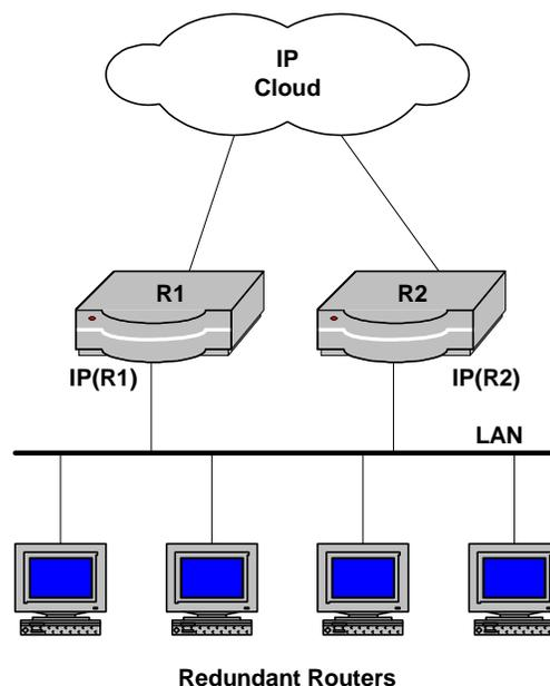
The virtual IP address IP(V1) is the real physical address of the router that is to be the primary router. In this example, IP(V1) will be equal to IP(R1). Router R1 is known as the *owner* of the virtual router.
