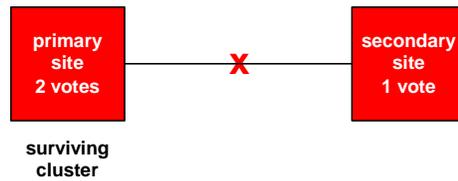
Should the secondary site fail, or should the communication link between the sites fail, the primary site will continue in operation since it has quorum. However, should the primary site fail, the secondary site will pause processing since it does not have quorum. Manual
