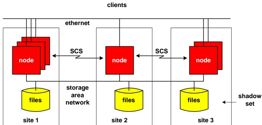
An application can be distributed across several nodes, and users can use any instance of an application on any node. To support shared-everything, OpenVMS clusters provide a Distributed Lock Manager that manages lock requests and a Connection Manager that manages the reconfiguration of the cluster should there be a failure. The Connection Manager ensures that there will not be two cluster subsets actively processing in a split-brain mode.
