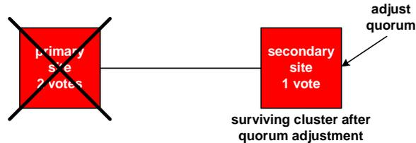
intervention is needed to change the quorum value to that of the votes held by the surviving site. At this point, the secondary system will take over processing. In a lights-out operation, the lights-out site should be the primary site since it may be difficult to get to it to manually adjust quorum.
