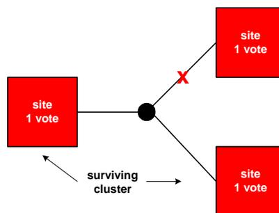
This configuration is often used in a two-site system with a third small quorum site. Alternatively, a quorum disk, not a member of a shadow set, can be connected to the SAN and can provide the
