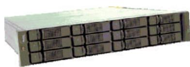
The disks can be arranged in any desired RAID array. RAID levels may be mixed within a single ftScalable array. The disks are hot-pluggable, and the dual RAID controllers provide a rolling upgrade capability for installing firmware upgrades without taking down the array.
