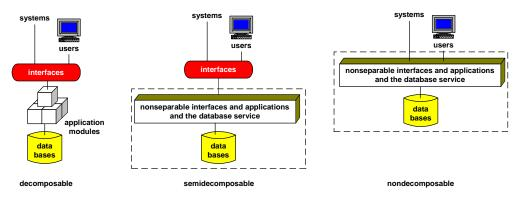
A decomposable system is one in which the presentation, application, and data layers can be easily separated. (The presentation layer is called the "interface" in the author's diagrams.)
