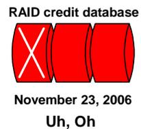
done was to insert the new drive and to rebuild it from the data on the other surviving drives. The full redundancy of the server would then be restored.
