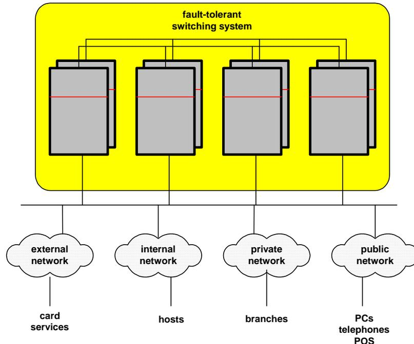
This system had fault tolerance fundamentally built into the box. Networking was integrated with the system. Failover times were virtually instant. It came completely configured with system management software with full automation support.
